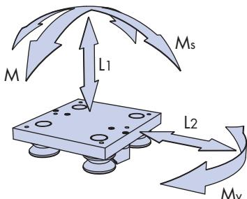
Load capacities apply to lubricated systems. For stainless steel systems loads are 25% lower. Contact Hepco for load and life of unlubricated systems.
