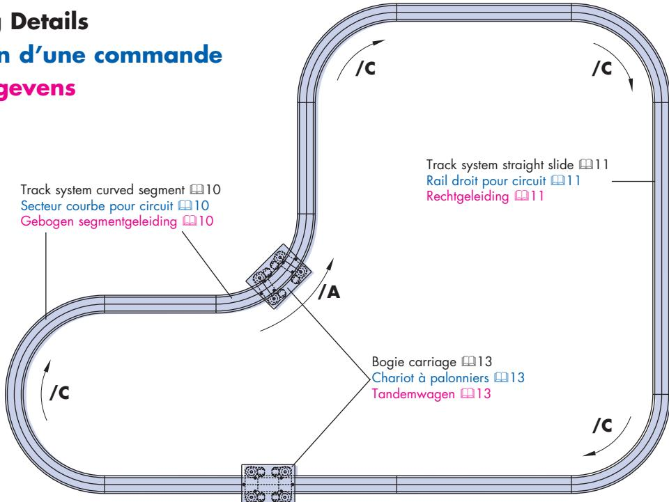
Please list part numbers of ring segments and straight slides in a clockwise sequence beginning at any point on the track system. Curved segments should be designated with a suffix "C" for a clockwise bend or an "A" for an anticlockwise bend.
